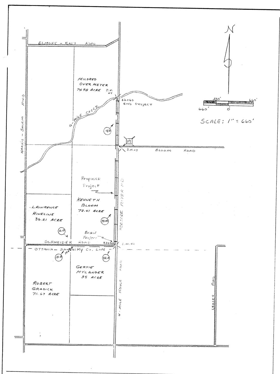
B.M.#1 TOP OF STEEL PIN UNDER METAL PLATE LOCATED IN CENTER OF 4-MILE HOUSE ROAD AND SCHNEIDER
